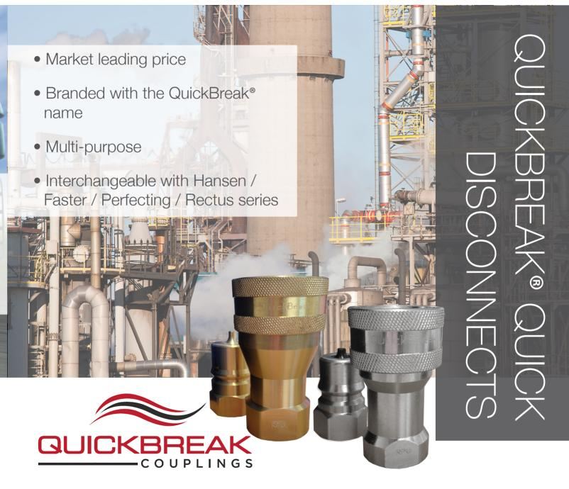
Consisting of couplings designed to ISO 7241-A (ISO A) and ISO 7241-B (ISO B) parts, the QuickBreak<sup>®</sup> multi-purpose poppet couplings are branded with the product code, material and size for track and traceability. Upon disconnection, the socket and plug valves seal instantly, automatically shutting off fluid flow to prevent leakage. On connection, the socket and plug valve push together, opening to permit free flow of fluid.
